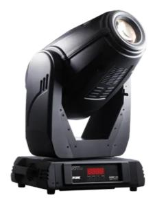
The ROBIN 300E Spot Classic is a punchy profile fixture with features such as linear zoom, a full package of rotating gobos, colour - gobo wheel including 4 colours and 5 static gobos and standard colour wheel. Up to 24 colour mixes can be achieved with a combination of the colour wheel and colour/gobo wheel.
